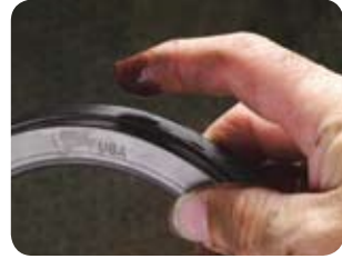
Lightly lubricate the OD and ID with the fluid being retained.
